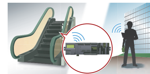
Programmable logic controllers and operator interfaces that enable remote monitoring and operations
