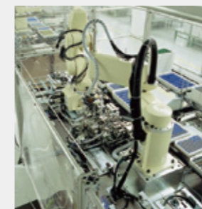
Robot control cellular production system at the Takino Plant
